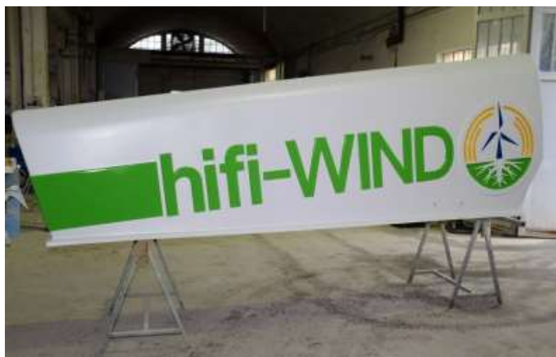
Carter of coverage for alternator of eolic tower.
